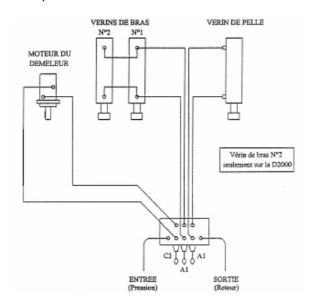
The distributer THROW DISTRI 2000 FIMAKS is equipped with an origin of independent hydraulic distributors to the tractor which is commanded by electrovans. This circuit needs only an alimentation with a return.
