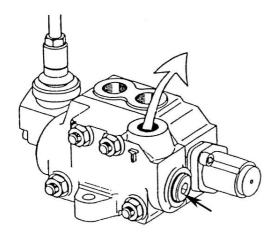
For adaptation of the hydraulic circuit with closed center
